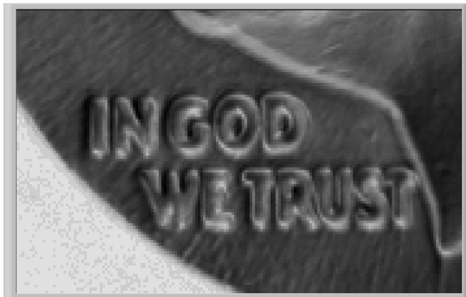
Figure 5.1-13: Backscatter plot of dime scan.
